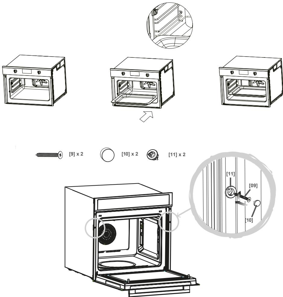
Once the oven has been lifted into place inside the appliance housing, locate the two holes in the casing of the oven and fix it into place using. [09], [10] и [11].
